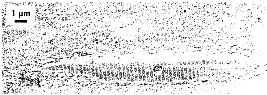
Figure 6. Adjacent layers of a crystal observed within its quenched matrix diverge from the central screw dislocation (Patel & Bassett, unpublished work).
